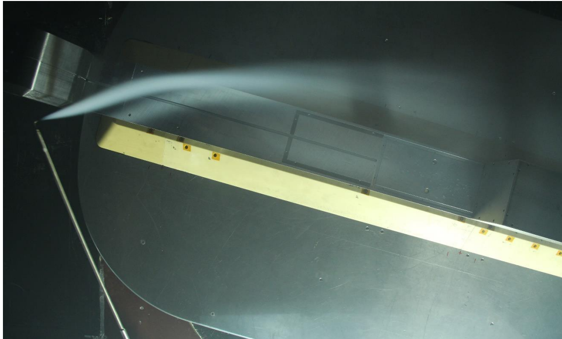
Top view: flow between upstream locomotive and downstream container
