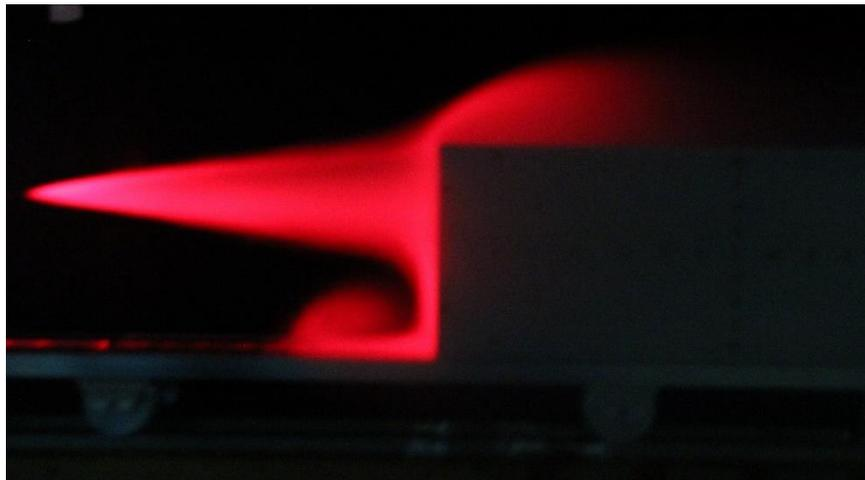
Figure 32: Highlighted smoke visualization over front windward (facing toward wind) surface
