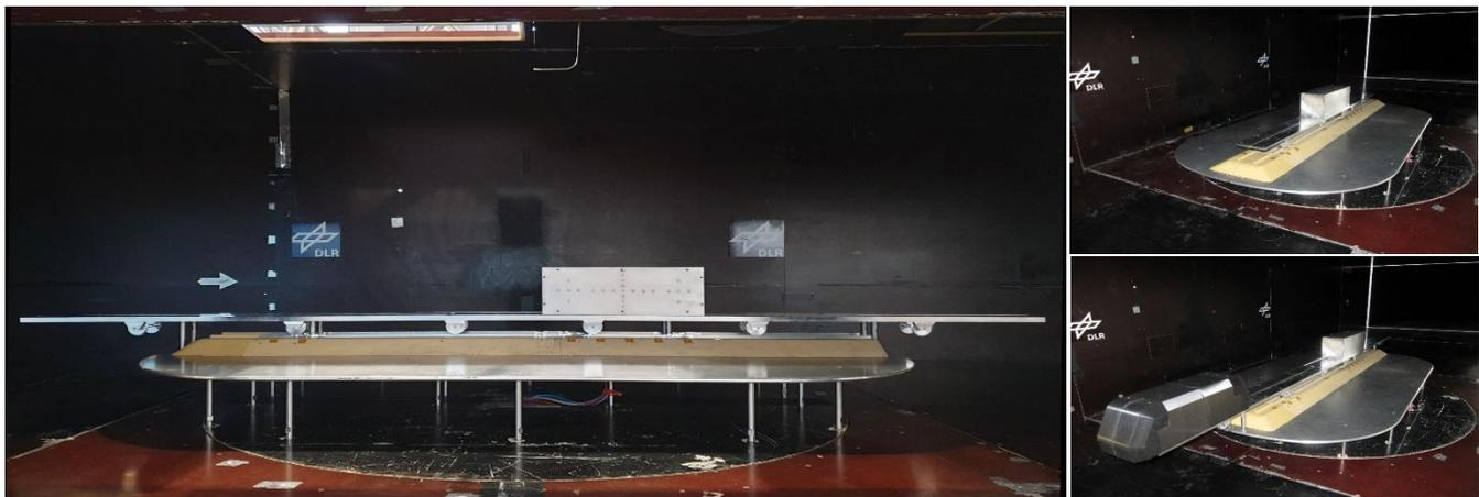
Figure 24: Photos of the FR8-LAB wind-tunnel experimental setup in different loading configurations
