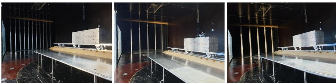
Figure 27: Turbulence configurations added upstream of the model test-position, left-right configurations: turb1, turb2 and turb3
