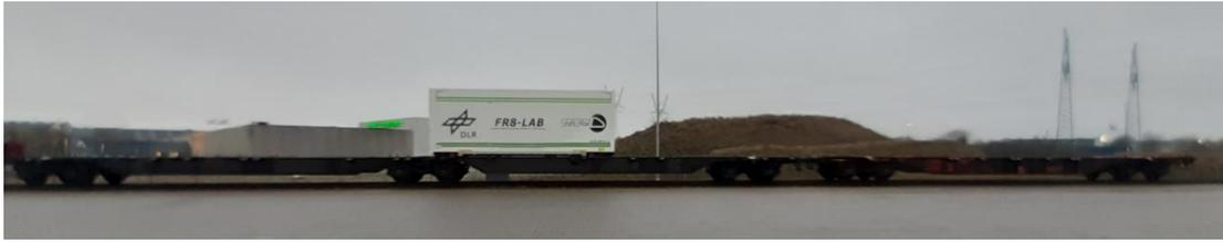
Figure 2: The FR8-LAB loaded on the test-wagon consist for the Great Belt Bridge experimental campaign
